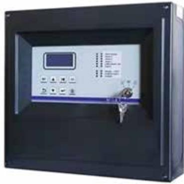
Central gas detection system with 8 zones to which it is possible to connect a toxic or explosive gas detector of proportional type 4-20mA. LCD display with 4 lines of 16 characters, membrane keyboard with protected access via mechanical key, 6 programmable relay outputs for pre-alarm, alarm and general fault with threshold management.
