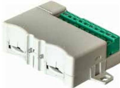
MMT is a 4÷20mA analogue input module for gas detectors and other device interfacement that use this standards. The module is compatible with new NOTIFIER panels series. Each MMT module use only one address of 99 available on loop. Microprocessed Module compatible with Notifier protocol, MMT is designed to manage a single detector. The address codification is achieved through decimal rotative switches.
