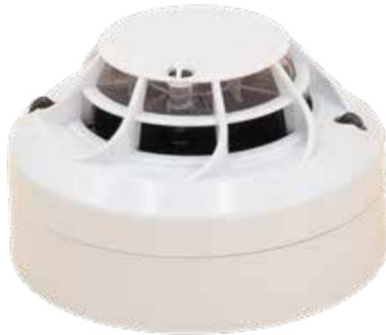
The multi-criteria multi-sensor MI-PTSE-S2I Photo Thermal detector uses thermal assistance to the core photoelectric smoke detector to give enhanced false alarm immunity and faster response to a wide range of incipient fires.
