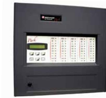
The PARK2000 carbon monoxide detection panels is specially designed for application in garages with 3 up to 5 CO detection zones. Each zone supports a maximum of 16 NCO100 detectors distributed over a line of up to 500m in length, with 1.5mm<sup>2</sup> cable section, twisted and shielded. They have a control module with an LCD screen that displays the alarm and fault levels of each zone and allows the reading of CO concentration per zone in sequential mode.
