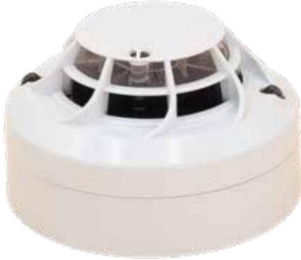
The MI-RHSE-S2I uses the same thermistor and microprocessor technology to provide an alarm when the rate of rise in temperature exceeds 10°C/ minute (typical) or if the temperature exceeds a threshold of 58°C (Response Class A1R).
