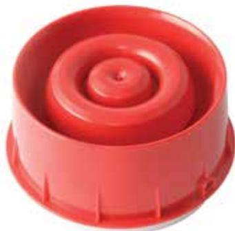
Honeywell Morley-IAS wall mounted sounder is installed in exactly the same manner as an intelligent fire detector. Common installation base (Part No. MI/B501AP/IV), which accepts any product within Honeywell Morley-IAS audible-visual product family, is installed at first fix. This common base is fitted with a shorting spring, enabling loop continuity to be maintained without having to install any Honeywell Morley-IAS audible-visual product.
