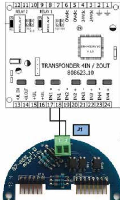
This interface was created to facilitate the connection to the ESSER by Honeywell transponder 808613/808623 since it provide already the EoL resistors needed to balancing the transponder input.
