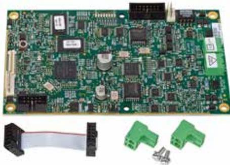
Plug and play card to expand the DXc2 panel capacity to 4 loops (396 sensors + 396 Modules)
