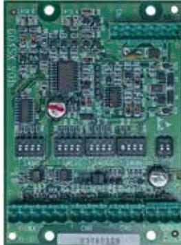
IIG4N is an addressable analog module with 4 inputs 4÷20 mA for interfacing with gas sensors with the same type of output.
