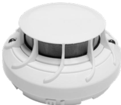
The MI-LZR-S3I high sensitivity, high gain amplifier based intelligent smoke sensor is a unique offering from Morley-IAS that provides extremely high sensitivity to fire conditions, by detecting the earliest particles of combustion. This is achieved by combining a patented optical chamber with advanced high power output IR LED diode and precision optics technology, which is matched with a unique superior high gain IR receiver amplifier, enhancing the sensitivity of the device.
