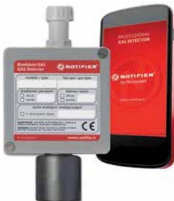
The gas detectors of the 700 Series PARK SS are specifically designed for gas detection in underground parking areas where such systems are required. The detectors are in IP55 enclosure and the two models available are for the detection of gasoline vapors, catalytic with sensitivity 0-100% of L.I.E. and CO (Carbon Monoxide) Electrochemical Cell with sensitivity 0 to 300 ppm.
