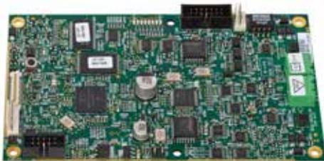
The DXc Network card order to connect panels together to create a DXc panel Network. It is required one Network card on each networking panel. The Honeywell Morley-IAS network is a peer to peer network with shared zones and keyboard, were each panel is equal in the network. The Network card is fitted in the control panel.
