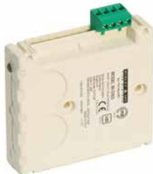
MI/DISO is intended to be spaced between groups of devices on a communication line to protect the line if a short circuit fault occurs. It automatically opens when the voltage in the communication line falls below a fixed threshold. If a short circuit fault occurs, the two isolators located around the device group where the fault occurred will sense the line voltage drop, open their switches and remove the devices from the rest of the line.
