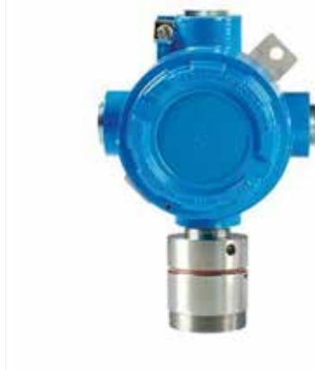
Chlorine / GAS / Butane Gas Detectors with Infrared Sensor. In EEx certified container, suitable for installations in classified AD-PE range 4-20mA proportional output. Measuring range 0 to 100% LEL.
