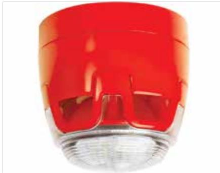
Combined acoustic and optical alarm signaling device, with IP65 Ingress rate protection enclosure is EN 54-3 & EN 54-23 compliant, in red housing, and offers a selection of 32 signal tones including the DIN tone and other country-specific tones. All tones comply with EN 54-3. Tone configuration takes place via a 6-pin DIP switch. Up to two different signal tones may be activated.
