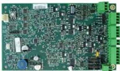
The System IO card provides a VdS DXc panel compliance interface to communicate with the required Fire Brigade equipment as part of the VdS compliant Fire System.
