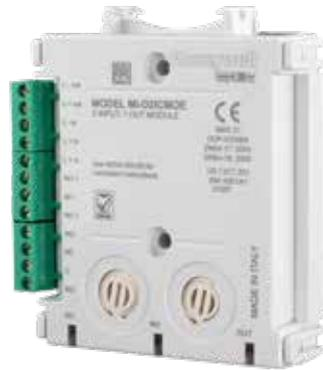
The MI-DCMOE optionally supervises the wiring to the load devices and, upon command from the control panel, switches an external power supply to operate these devices. It also has built-in short circuit isolation capability.
