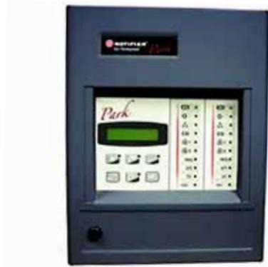
The PARK2000 carbon monoxide detection panels is specially designed for application in garages with 1 up to 2 CO detection zones. Each zone supports a maximum of 16 NCO100 detectors distributed over a line of up to 500m in length, with 1.5mm<sup>2</sup> cable section, twisted and shielded. They have a control module with an LCD screen that displays the alarm and fault levels of each zone and allows the reading of CO concentration per zone in sequential mode.
