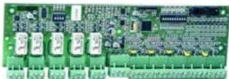
The MCX-55ME card can be used with all addressable NOTIFIER fire Panels either with CLIP protocol (1-99) that Advanced protocol (1-159). It hold on board 5 monitor modules 5 and 5 control modules with relay with voltage free contacts.
