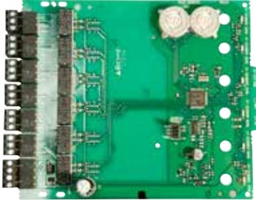
The CR-6 consists of six Form C relays.
