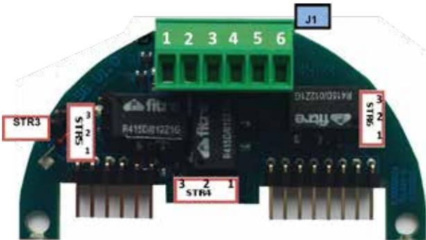
The 3-relay interface gives the possibility to have a dry contact for each single event: alarm, pre-alarm and fault.
