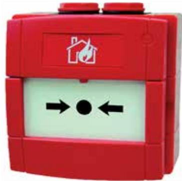
The outdoor MCP is an IP 67 sealed product. The enhanced environmental protection allows the unit to be installed in many external environments where water and dirt are likely to be present, making it a true waterproof and outdoor product. The manual call point has a unique 'plug and play' concept designed specifically to reduce installation time. The product utilizes a special terminal block, where all initial installation cabling is terminated.
