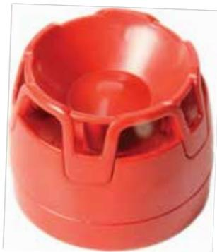
The acoustic alarm signaling device with IP65 ingress rate protection enclosure is EN 54-3 compliant, in red housing, and offers a selection of 32 signal tones including the DIN tone and other country-specific tones. All tones comply with EN 54-3.
