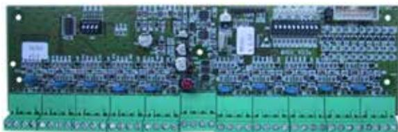
The MMX-10ME multi-module can operate with all addressable NOTIFIER Fire Panels either with CLIP protocol (1-99) or ADVANCED protocol (1-159).
