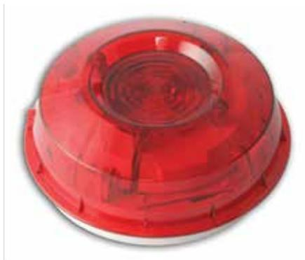
The wall mounted strobe is installed in exactly the same manner as an intelligent fire detector. A separate, common installation base (Part No. MI/B50IAP/IV) which accepts any product within Honeywell Morley-IAS audible-visual product family, is installed at first fix. This common base is fitted with a shorting spring, enabling loop continuity to be maintained without having to install any audible-visual product.
