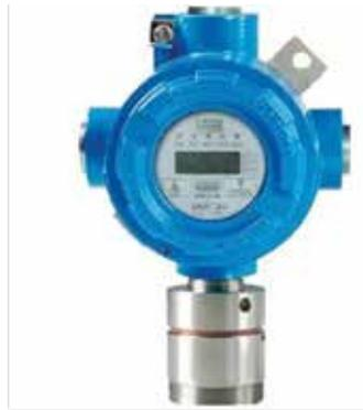
Methane / Ammonia detectors with Infrared sensor and LCD display in EEx certified container. D. Proportional output 4-20mA. Measuring range 0 to 100% LEL. Zero Tracker to counter possible drifts.
