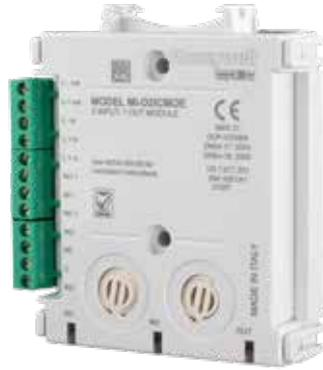
The MI-D2ICMOE provide supervision of one input circuits respectively from external devices; it also provides an unmonitored single pole volt-free changeover contact for external devices. All modules feature a built-in short circuit isolator.
