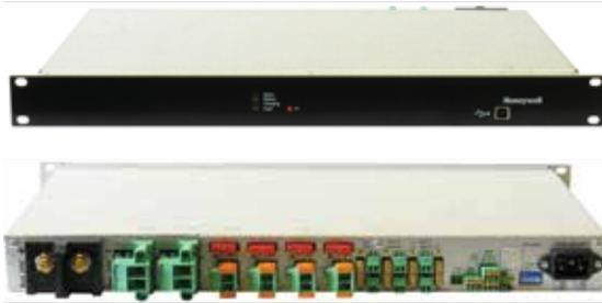
The Emergency Power Supply acts as a battery charger and control device for 24V DC external back up batteries in accordance with EN 54-4+A1+A2 standards. The front panel includes LED indicators, control push button and USB socket, allowing control and test of power supply operating parameters.
