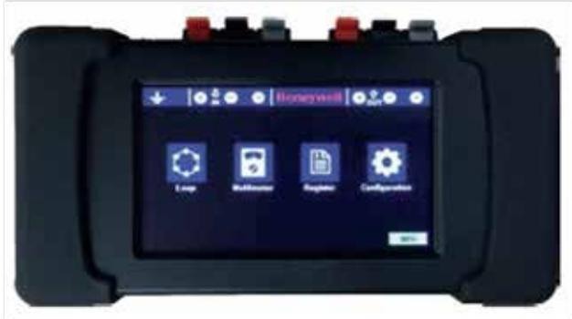
Intelligent loop diagnostic hand tool helps in the start-up installation process and maintenance works of Fire Alarm Systems. The tool visualizes Information on the Screen with Color graphic symbols. It allows to perform a loop diagnostic before connect to the fire alarm panel and verifies loop device addresses for errors or possible double addressing.
