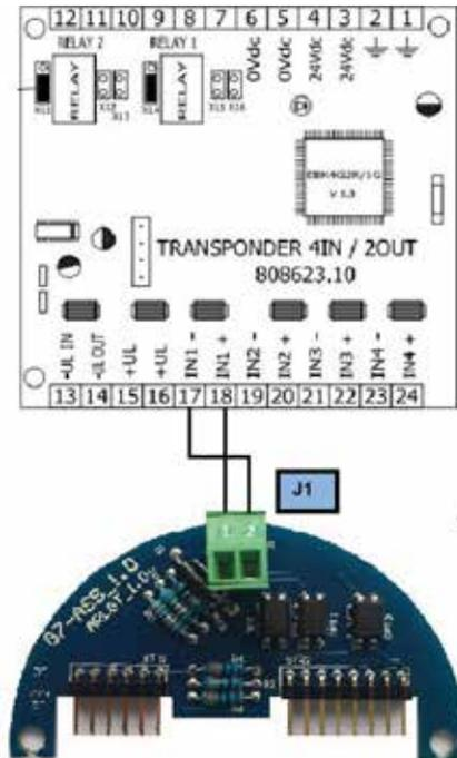
The interface can separately manage the pre-alarm, alarm and fault with open-collector outputs.
