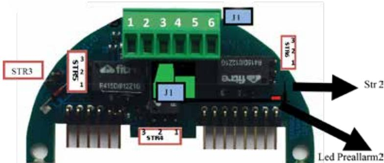
The 3 relays interface provide a free of voltage relay for each single event: alarm, prealarm, prealarm 2 and detector fault.
