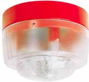
Optical signaling device compliant with EN 54-23 for wall and ceiling mounting with white strobe color and flat base. The signaling device is suitable for square signal ranges W-2.4-9.0 and cylindrical signal ranges C-3-9.5 / C-6-9.5 / C-9-9.5.
