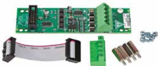
The RS232 port card provides the external connection of peripherals with a proprietary protocol to give and control external equipment.
