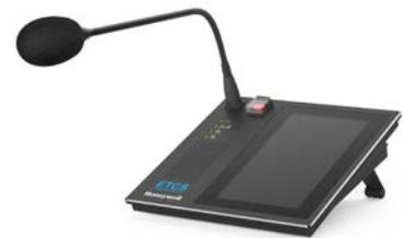
*For display and operation, the Ethernet Touchscreen Call Station (ETCS) offers a 7" touchscreen with a user-friendly interface.*
