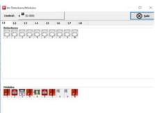
In the event of an alarm or any other event, we can make a graphic representation, in real time, of the condition of the sensor (ID3000) or temperature values in the zone (Sensa). In this way, we can quickly evaluate the status of the alarm and carry out actions on the sounder modules, even before the control panel performs the evacuation process.
